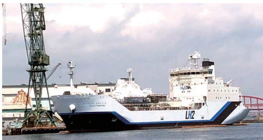
Fig. 8 Liquefied hydrogen carrier under outfitting (May 2020)
